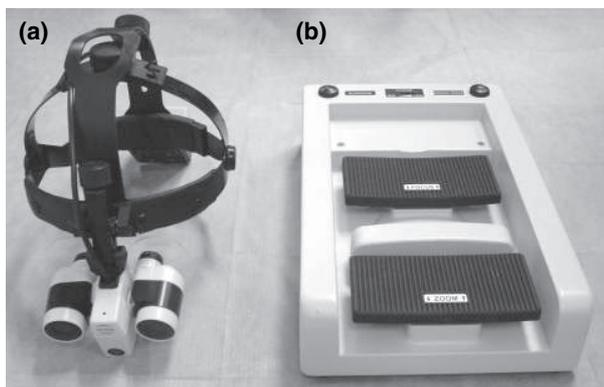
**Figure 1** The Varioscope® AF3 is a head-mounted surgical telescope with automatic focusing and continuous zoom magnification from 3.6× to 7.2× that can be operated using a footswitch. This device refocuses if the working distance changes, and the surgeon has almost unlimited mobility without any corresponding loss of sharpness in the obtained three-dimensional images. (a) Head-mounted surgical telescope. (b) Footswitch for focusing and zoom magnification.
