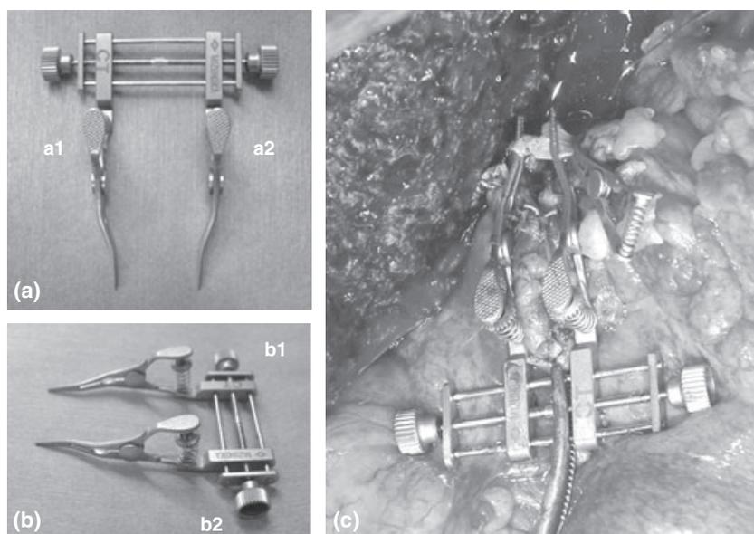
**Figure 2** The microvascular double clamp type A-II device comprising 4.2 cm long bulldog clamps and weighing 17 g. By rotating b1 or b2, the distance of the two tips can be freely adjusted from 0 to 25 mm. By rotating a1 and a2, the pressure required to open the tips can be adjusted from approximately 40–250 g. (a) Frontal view. (b) Oblique view. (c) Use of the device during end-to-end anastomosis of the hepatic artery for living-donor liver transplantation with a right lobe.
