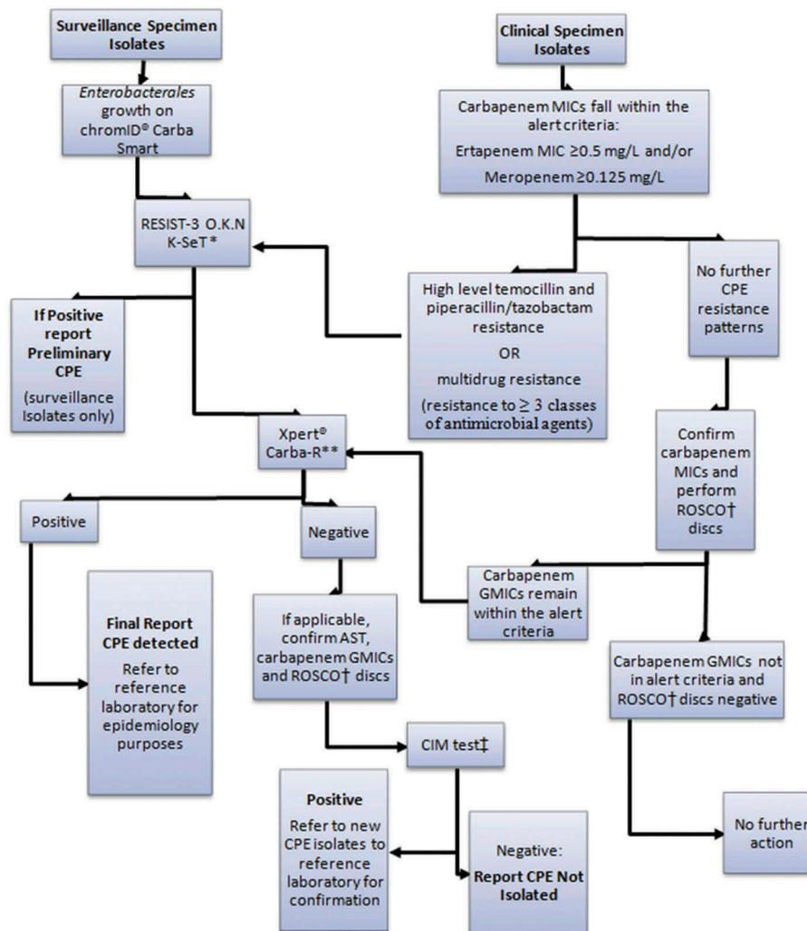
Figure 1. CPE Detection Algorithm.
