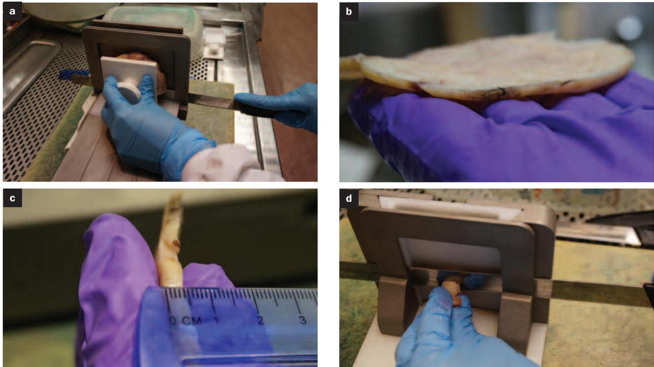
**Fig. 2.** **a)** TruSlice Digital grossing of a large lipoma, using an immobilising plate; **b)** Transverse slice of lipoma grossed (as in Fig. 2a), demonstrating the uniform perpendicular result achieved; **c)** Lipoma slice (as in Fig. 2b), demonstrating the uniform thickness of 4 mm, across the entire length; and **d)** A sebaceous cyst grossed using the TruSlice device
