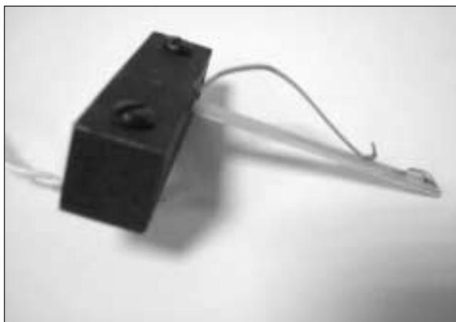
**Fig. 2.** Close up view of impedance probe assembly showing the electrodes on the extreme right of the picture.
