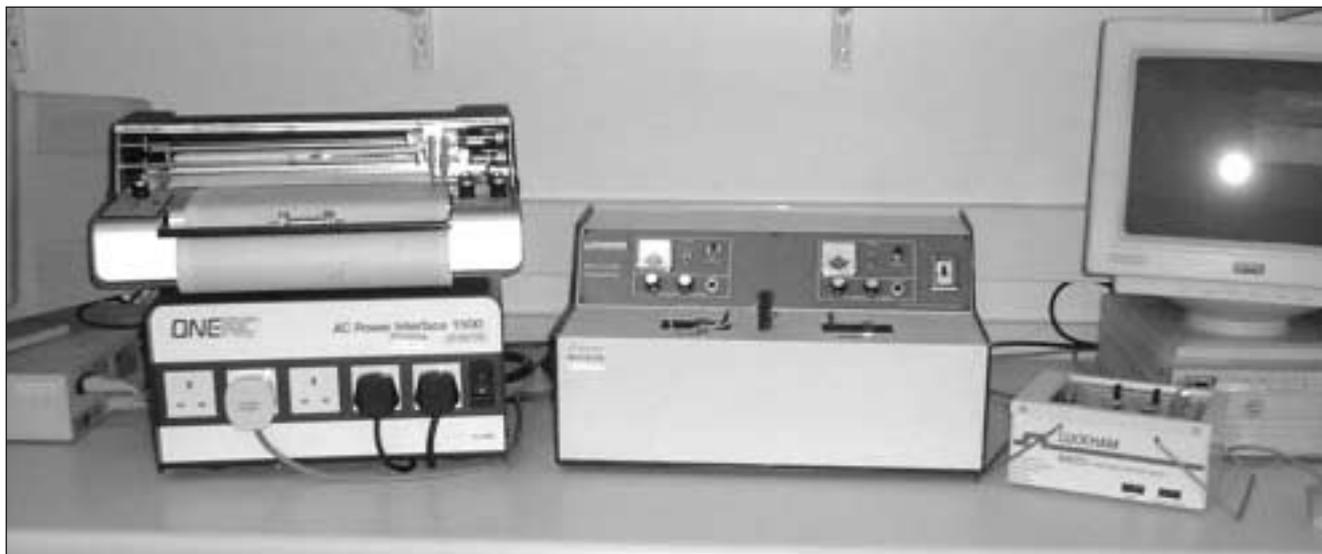
**Fig. 1.** Photograph showing equipment used, with the Chronolog 540 aggregometer (centre), stabilised power supply with chart recorder on top (left) and a water bath for pre-incubating samples, reagents and probes (right).
