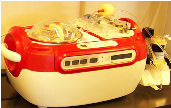
Figure 1 Portable perfusion pump. The HeartPort© System is a modified version of the LifePort© System (Organ Recovery Systems©, Itasca, IL, USA), designed for kidney graft perfusion and preservation. Heart grafts are suspended inside a sterile cassette and subjected to retrograde perfusion with 1 L asanguineous preservation solution (KPS-1©, Organ Recovery Systems©, Itasca, IL, USA). The perfusate is cooled to 4 °C by a heater exchanger, oxygenated by oxygenator (Minimax Oxygenation System©, Medtronic Inc, Minneapolis, MN, USA), and recirculated by means of a pulsatile roller pump. The system includes a data report unit that allows for temperature, perfusion pressure, and flow to be continuously recorded.
