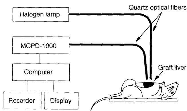
**Fig. 1** Block diagram of in vivo near-infrared spectroscopy apparatus
