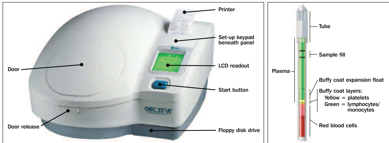
Fig. 1. (Left) QBC Star haematology centrifugal analyser. Fig. 2. (Right) Diagram of the QBC Star tube.
