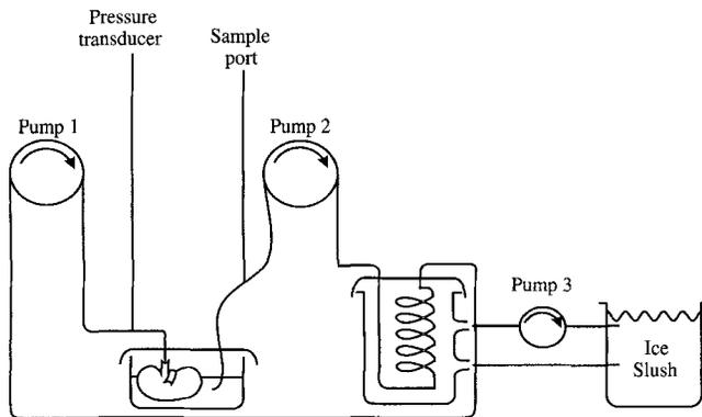
**Fig. 1** The renal artery is perfused with UW solution via pump no.1, while the effluent from the vein is collected by pump no.2 and re-circulated. This forms a closed system of 500 ml of UW solution. Temperature is controlled at 4–8 C by a heat exchange system, serviced by pump no. 3. The system is maintained at 45–60 mm of Hg pressures. Sample port on 'venous' limb allows measurement of GST and proteases. Pressure transducer on 'arterial' limb enables measurement of IRVR and flow rates
