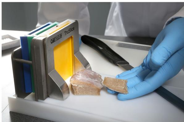
**Figure 2.** Showing the use of the TruSlice device sectioning tissue at a defined thickness with accuracy and precision.
