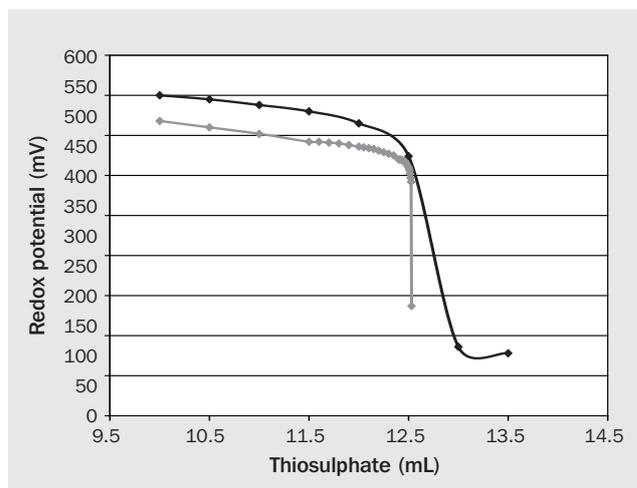
**Fig. 2.** Hypochlorite titration. Sodium thiosulphate ( $\text{Na}_2\text{S}_2\text{O}_3$ ) is added until a significant drop in redox potential is observed (black curve). Repeated titration using smaller and more precise increments (grey curve) determines commercial hypochlorite concentration to be 2.33%, or approximately 40% of labelled concentration.
