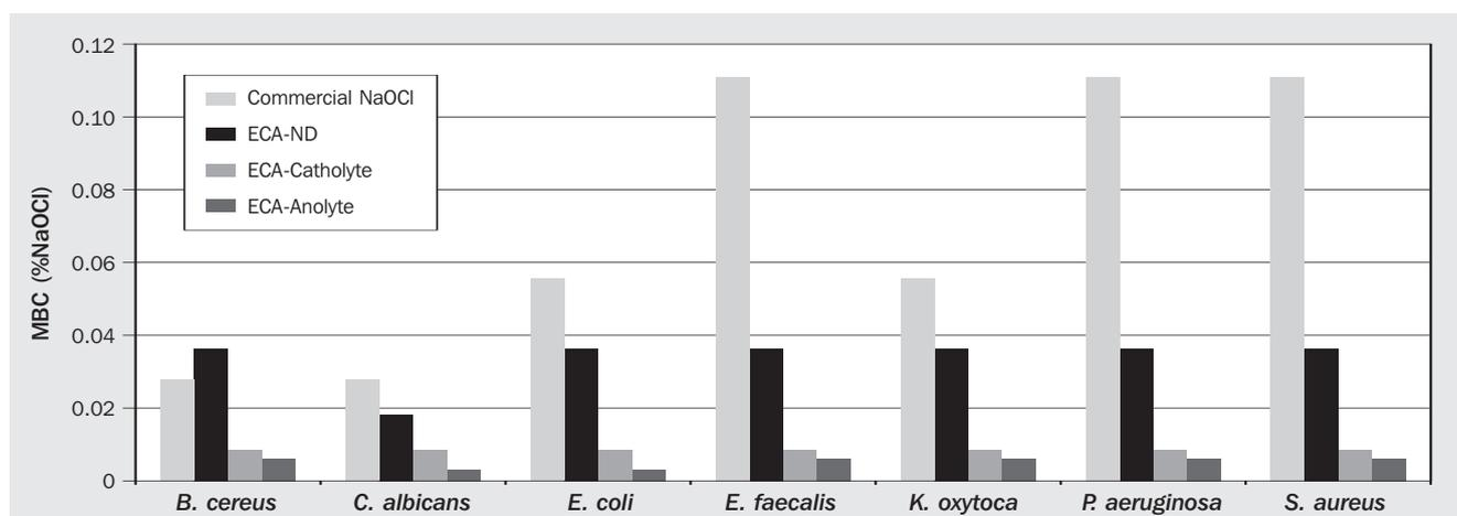
Fig. 5. Minimum bactericidal concentration. The MBCs determined by this study for the various solutions and organisms tested are compared. The lowest MBC being the most efficient, the anolyte and catholyte solutions are significantly more efficient disinfectants than the ECA-ND solution or the standard hypochlorite solution of equal concentration.
