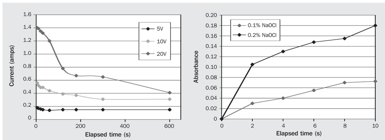
Fig. 4. Time vs. current and time vs. absorbance – ECA-ND (single) chamber, 292.5 nm.
