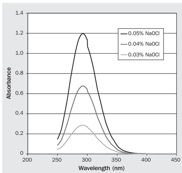
**Fig. 3.** Wavelength scan. Absorbance of commercially available hypochlorite is recorded every 0.5 nm from 250 nm to 400 nm to determine the optimal wavelength for quantitative measurement. 292.5 nm was used for all hypochlorite determinations in this study.
